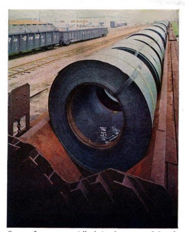
Concave flatcars are specially designed to carry coiled steel.
