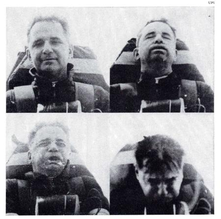
Stapp comes to quick, body-punishing halt after racing rocket sled down rails.
