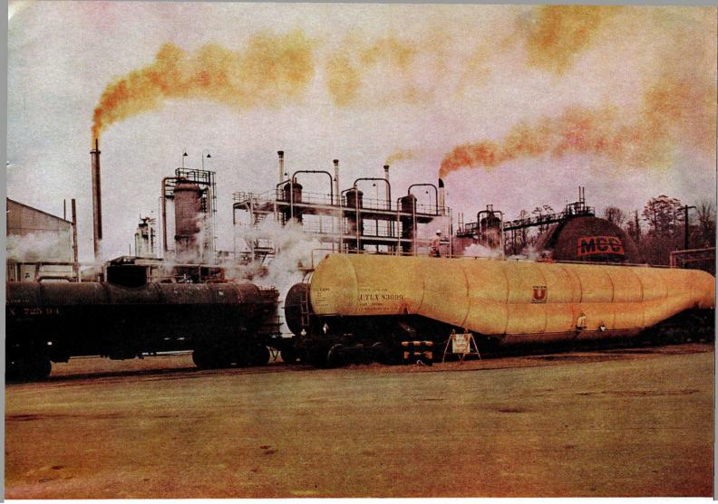
The "Pregnant Whale," a jumbo tank car with 50,000 gallon capacity, dwarfs standard-sized 10,000 gallon tank cars.
